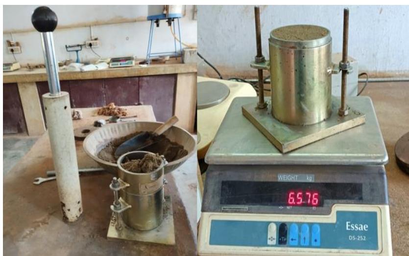
Figure 3: Proctor compaction test apparatus
