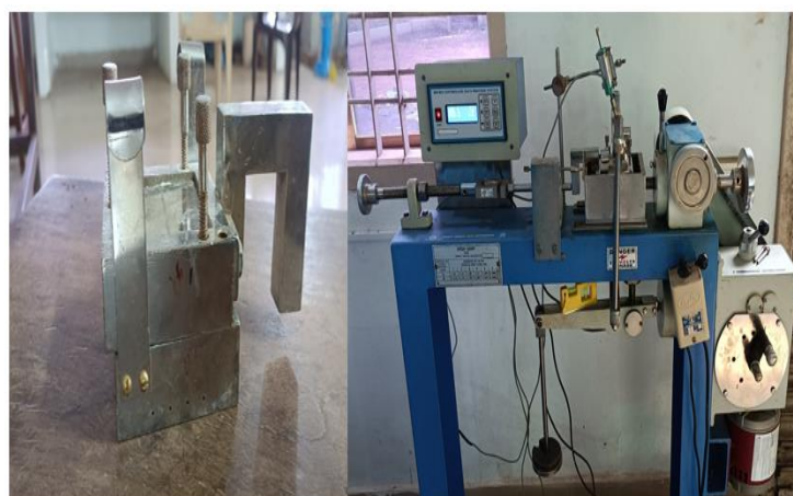
Figure 4: Direct shear test apparatus
