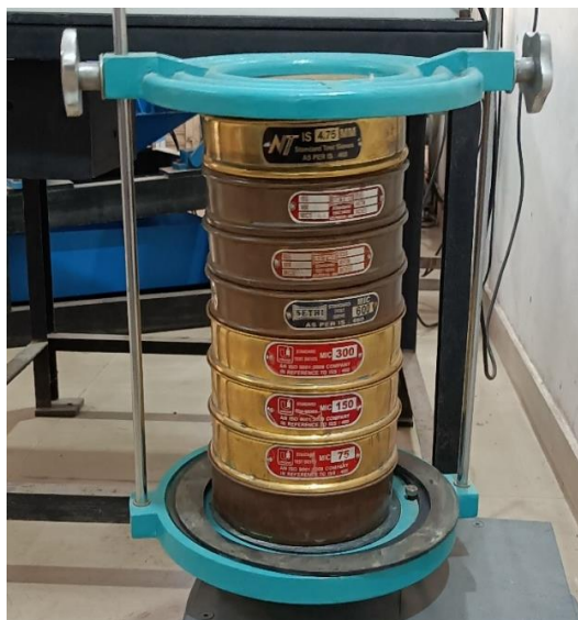
Figure 2: Sieve Analysis Test apparatus
